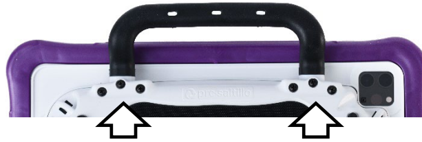
Via Pro: Remove six screws
