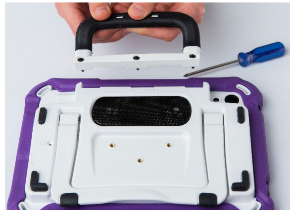
Via Mini: Remove three screws
