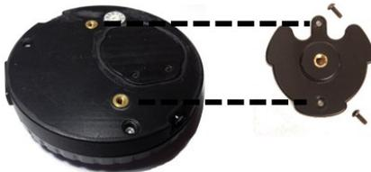
2. Insert the screws in the holes and tighten.
