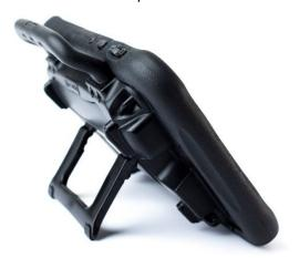
The stand is adjustable. It will remain in any position you move it to. To position the device at an angle for easy viewing of the screen, grab the rounded area on the stand's bottom support and pull away from the back of the device.
