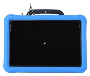
1 Power button: Press and hold to turn the device on or off
