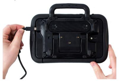
4. The charging LED beside the charging port should be flashing while the batteries are charging and will glow steadily when the batteries are fully charged.
